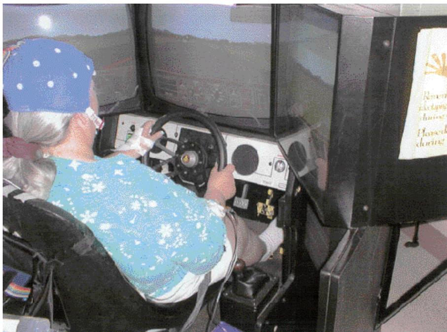
Figure 2—Atari Research Driving Simulator.
